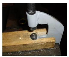
This picture shows the mock-up knife in the hammer rivet set jig. I supported the blade with my left hand while using the right hand to gently hammer the upper set. I gave it a couple of taps, checked the tightness of the blade in the scales and then repeated on the other side. The process repeated until the feel of the blade was right.
