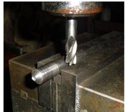
If you have ever used the drill bits that have a more-or-less triangular end, you know how well they work in a drill chuck. The same idea can be applied to the spinners. Get some scrap hex material (a big hex nut would do in a pinch), drill a  $\frac{1}{2}$ " hole in the center, add a couple of set screws and you get the jig shown here.
